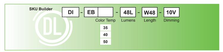
Example: DI-EB50-40L-W48-10V = Diode, 120 Volt, EMERY™ BEAM, 5,000° CCT, 4800 Lumens, 48" length.
